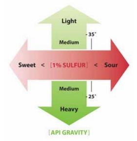
Figure 2. Oil Density and Sulfur Content Scale. Source: Bureau of Ocean Energy Management
